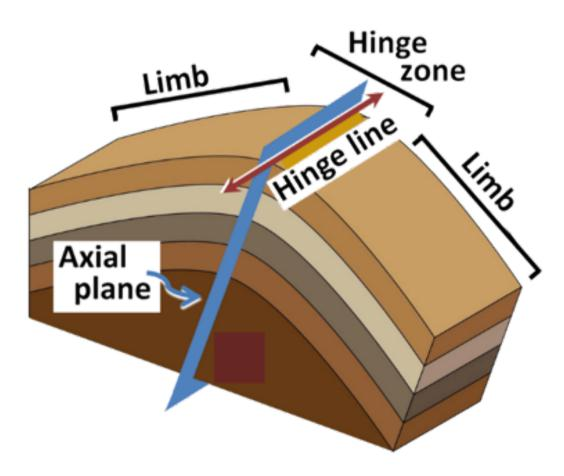
The Pinta Dome, Navajo Springs & East Navajo Springs gas fields characterized by: (i) anticlinal features; (ii) favorable reservoir rocks and (iii) impermeable caprock traps.
